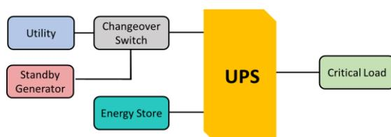
Figure 1. Generic UPS, Utility and Standby Generator arrangement.
