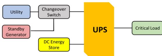
Figure 4. Electrically-coupled UPS Block Diagram
