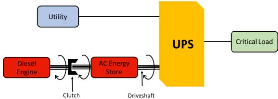
Figure 3a. Mechanically-coupled UPS with Standby Engine (DRUPS) Block Diagram.
