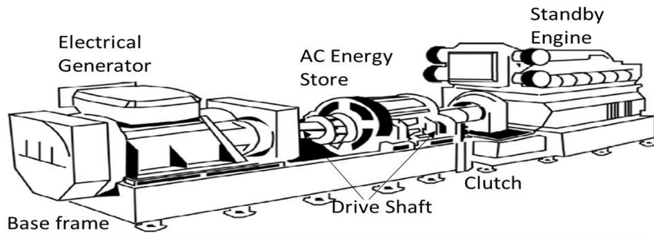
Figure 3b. Typical Mechanically-coupled DRUPS base frame layout
