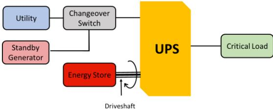
Figure 2. Mechanically-coupled UPS Block Diagram
